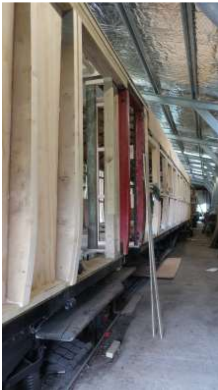
Fantail: above – Bill paints a seemingly “endless” supply of seat frames; left outside & inside – wall frames standing tall, roof cladding begun; below – side view - window frames in, and start of wall cladding. In the left foreground – the two green “boxes” are Gabriel’s water tanks
