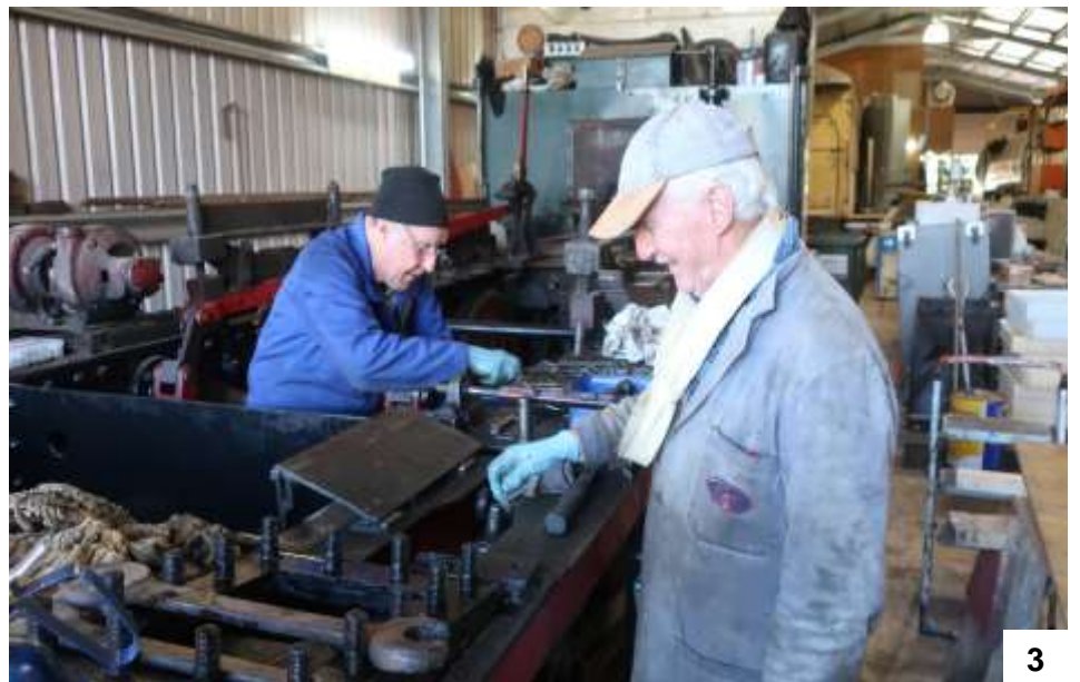
Below: David and Mike – setting the slide valves in Gabriel’s valve gear David is standing inside the wheelbase, & the cab stands upright beyond.
