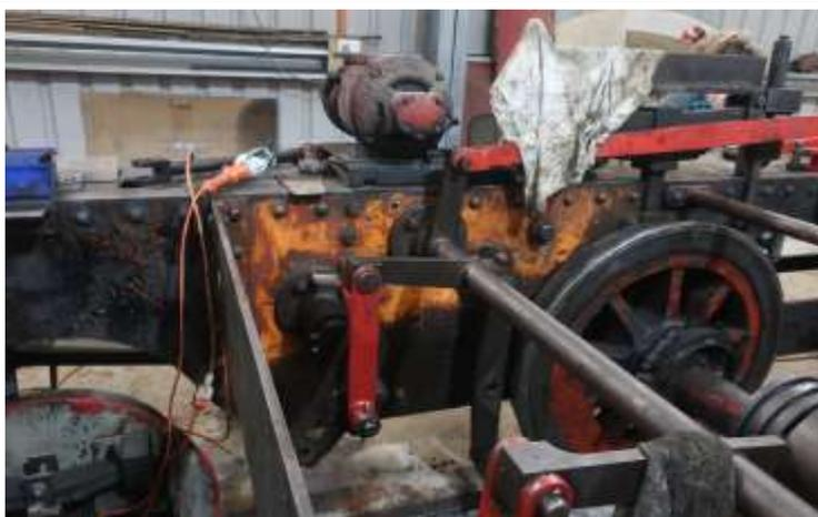
Inside Gabriel's chassis: Stevenson valve gear. Major components: reversing rod (red horizontal bar). Expansion link & lifting link (red vertical bar & curved black link next to it). On the axle - part of the eccentrics.
