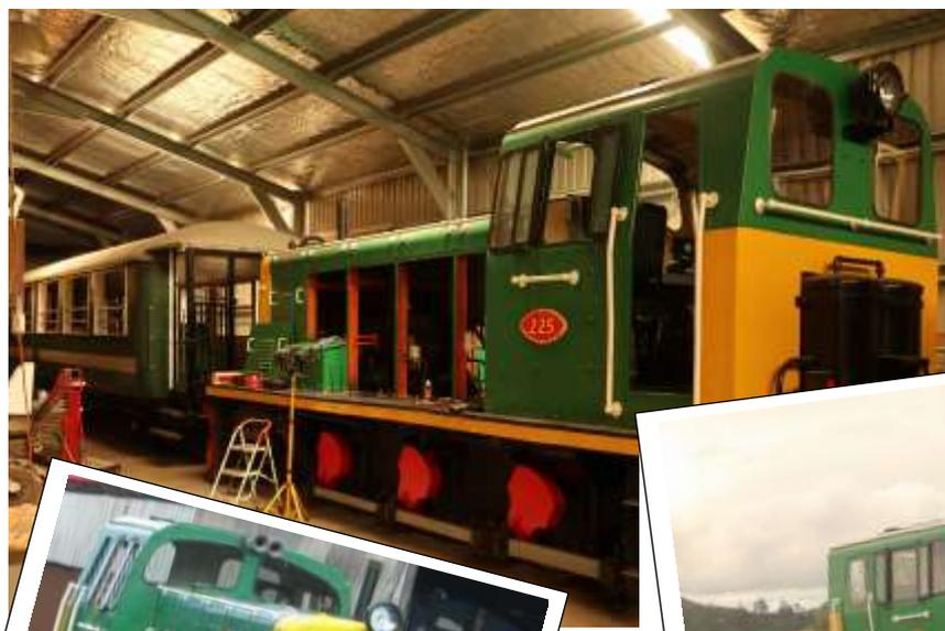
DSA225 has been out of service for some time. The following problems have been addressed to refurbish this loco and get her ready for hauling passenger trains again: fuel injector pump, starter motor and ring gear. The fluid clutch had to be removed and refitted to get the flywheel off to replace the ring gear, and a new Bendix was fitted. All this between maintenance for our working locos! Thank you, Frits. See below left
