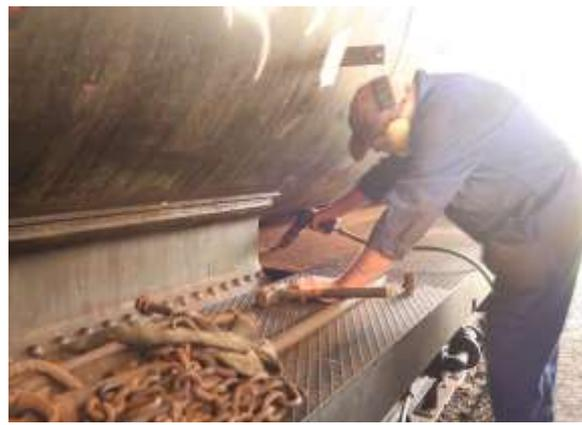
Many months of patient de-rusting of the fuel tanker by Morris McLeary has been taking place. He'd using rust treatment paint as he works. The mystery pipes (p1) are brake pipes which will soon be fitted to the tanker.
