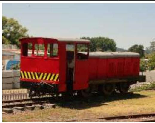
Sweetie has a new coat of paint to greet our visitors. Built 1896 at Addington loco works as a 0-6-2, Fa 9 steam engine; now 0-6-0; used to work at AFFCO
