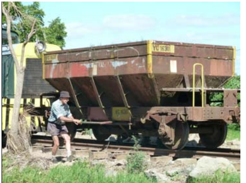
(Above) All the sleepers and spikes are back in place and await ballasting. (Below) Graham Winterbourn lays the ballast as the ballast wagons come into service for the first time
